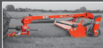
Gyrodine® swivel hitch allows over 90° turns for outstanding maneuverability
