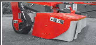
Constant Float® suspension closely follows ground to reduce missed crop
